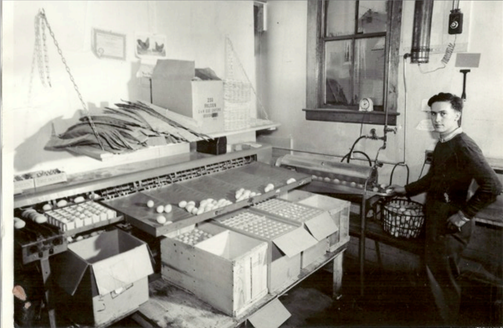
Richard Boutwell - loads eggs onto washer section of automatic grader
